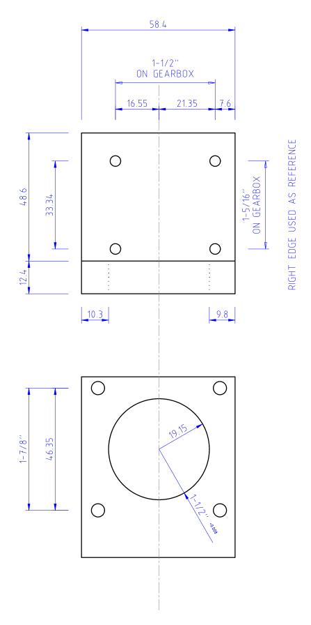
Figure 4: Declination mounting bracket. Front and top views. 1:1 scale.
