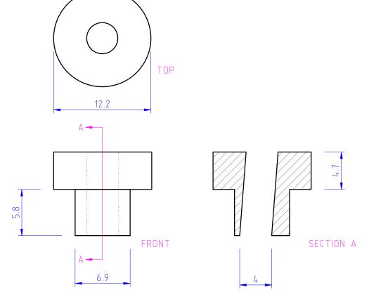
Figure 12: New collar, before changes. 3:1 scale.
