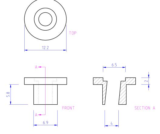
Figure 13: New collar, after changes. 3:1 scale.
