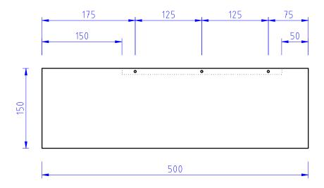
Figure 1: RA worm-wheel sun shield. 1:5 scale.
