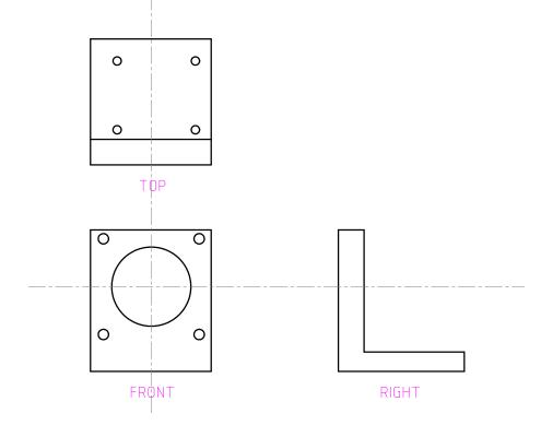
Figure 3: Views of the declination mounting bracket.
