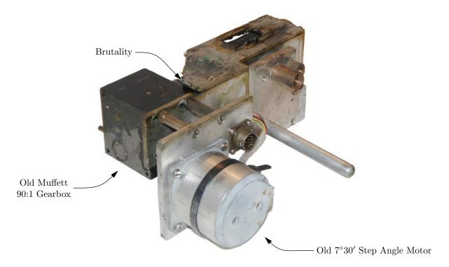
Figure 9: The worm cover was brutally bent out of the way.
