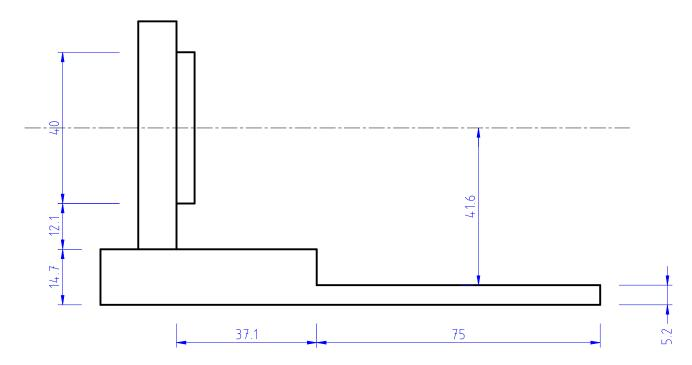
Figure 7: Motor assembly. Right view. 1:1 scale.
