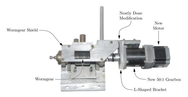
Figure 10: The new declination motor attached to the old motor assembly.
