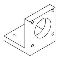
Figure 2: The motor mounting bracket.
