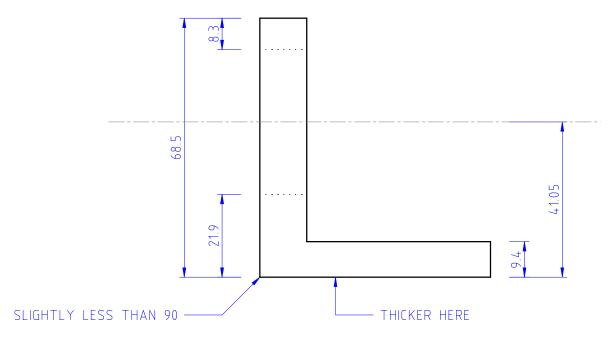
Figure 5: Declination mounting bracket. Right view. 1:1 scale.
