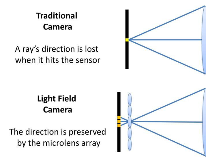
A light field camera captures 3-D data from a single image. This is because a microlens array, consisting of thousands of tiny lenses, splits rays coming from different directions onto different pixels. Knowing a ray's intensity and direction means from a single raw image we can digitally refocus, change viewpoint, aperture, and estimate depths within a scene. These abilities come at the expense of spatial resolution.
