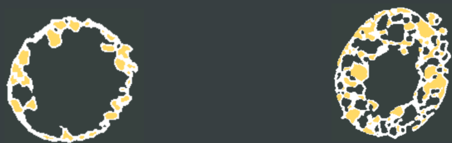
Fig 3. Salt (yellow) and binder (white) location in the granule of powder A and B, respectively.
